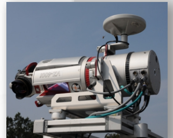
horizontal setup for, e.g. road surface scans
