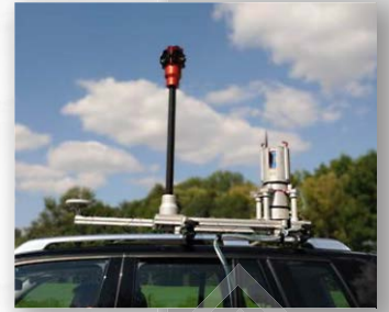
vertical scanner setup with additional panoramic camera system
